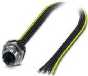
Flush-type connector, Power, 4-position, Socket, M12, S power, Rear mounting, M16 x 1.5, Individual wires, cable length: 1 m, 1.31 mm 2 , UL/cUL stranded hook-up wire
