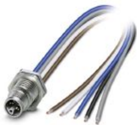
Flush-type connector, Power, 5-position, Plug, M12, L - Power, Rear mounting, M16 x 1.5, Individual wires, cable length: 1 m, 2.50 mm², PEX litz wire
