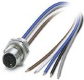
Flush-type connector, Power, 5-position, Socket, M12, L-coded, Rear mounting, M16 x 1.5, Individual wires, cable length: 0.5 m, 2.50 mm 2 , PEX litz wire
