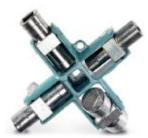
Control cabinet keys made of metal for all the usual closures: Two-way key bit 3-5 mm, square 5,6,7-8,9-10 mm, triangle 7,8-9,10-11 mm, special 6 mm
