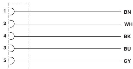
Contact assignment of the M12 socket
