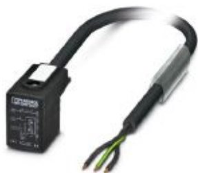
Sensor/actuator cable, 3-position, PVC, black RAL 9005, free cable end, on Valve connector BI (11 mm), with 1 LED, connected with Z diode, cable length: 3 m
