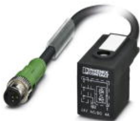
Sensor/actuator cable, 3-position, PUR halogen-free, black-gray RAL 7021, Plug straight M12, A-coded, on Valve connector BI (11 mm), with 1 LED, connected with Z diode, connected with Z diode, cable length: 0.6 m
