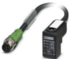
Sensor/actuator cable, 3-position, PUR, black-gray RAL 7021, Plug straight M12, A-coded, on Valve connector CI (9.4 mm), with 1 LED, connected with Z diode, connected with Z diode, cable length: 0.3 m
