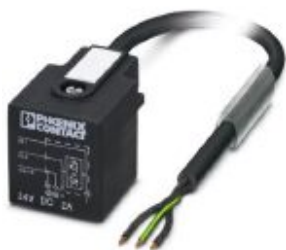
Sensor/actuator cable, 3-position, PUR halogen-free, black-gray RAL 7021, free cable end, on Valve connector A, with 1 LED, connected with Damping diode, cable length: 5 m
