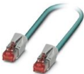
Assembled Ethernet cable, CAT5e, shielded, 2-pair, AWG 26 stranded (7-wire), RAL 5021 (water blue), RJ45 connector/IP20 on RJ45 connector/IP20, line, length 0.3 m
