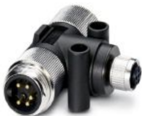
Bus system T-connector, DeviceNet™, 5-position, unshielded, Plug straight 7/8"-16UNF, on Socket straight M12, coding: A and Plug straight 7/8"-16UNF, Parallel distributor
