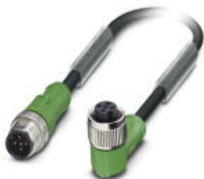
Sensor/actuator cable, 5-position, PUR halogen-free, black-gray RAL 7021, shielded, Plug straight M12, A-coded, on Socket angled M12, A-coded, cable length: 1 m, Shield on PIN5
