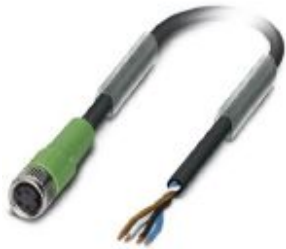
Sensor/actuator cable, 4-position, PVC, black RAL 9005, free cable end, on Socket straight M8, cable length: 10 m
