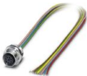
Sensor/actuator flush-type socket, 8-pos., M12, front/screw mounting with Pg9 thread, with 1 m TPE litz wire, 8 x 0.25 mm 2 , high-grade steel version, molded version
