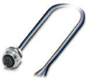
Sensor/actuator flush-type socket, 4-pos., M12, A-coded, front/screw mounting with Pg9 thread, with 1 m TPE litz wire, 4 x 0.34 mm 2 , stainless steel version, molded version
