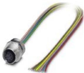
Sensor/actuator flush-type socket, 8-pos., M12, A-coded, front/screw mounting with Pg9 thread, with 2.0 m TPE litz wire, 8 x 0.25 mm 2
