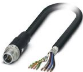
Hybrid cable, Ethernet hybrid CAT5 (100 Mbps), 8-position, Plug straight M12 SPEEDCON / IP67, coding: Y, on free cable end, cable length: 15 m, Power with Ethernet (PWE)
