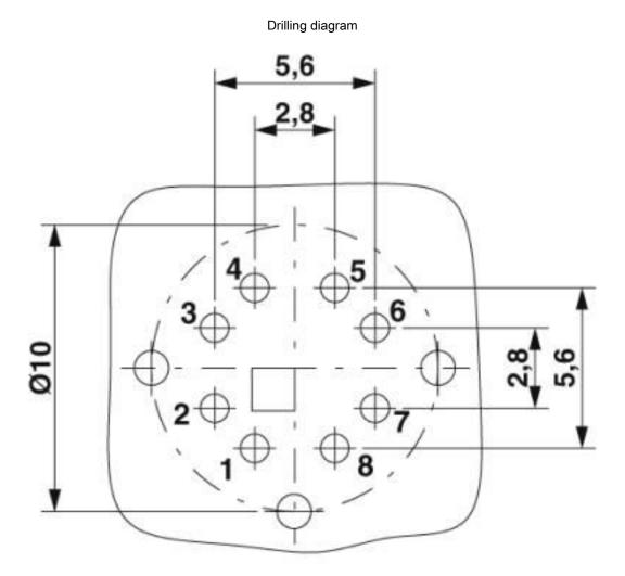
Soldering pad geometry
