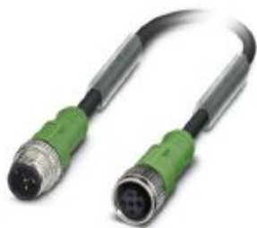
Sensor/actuator cable, 3-position, PUR halogen-free, black-gray RAL 7021, Plug straight M12, coding: A, on Socket straight M12, coding: A, cable length: 5 m, For valve connector
