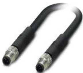
Sensor/actuator cable, 4-position, PUR, black RAL 9005, Plug straight M5, A-coded, on Plug straight M5, A-coded, cable length: 0.2 m
