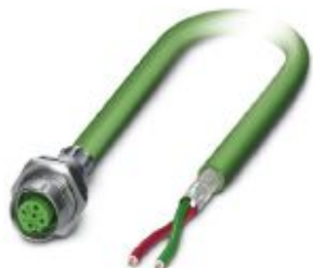
Bus system flush-type plug, PROFIBUS, 2-pos., M12, shielded, green outer sheath, B-coded, rear/screw mounting with M16 thread, with 2 m bus cable, 2 x 0.25 mm 2
