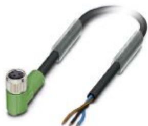
Sensor/actuator cable, 3-position, PVC, black RAL 9005, free cable end, on Socket angled M8, cable length: 5 m
