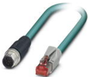
Assembled Ethernet cable, shielded, 4-pair, AWG 26, stranded (7-wire), RAL 5021 (aqua blue), M12 plug to RJ45 plug/IP20, line, length 15 m
