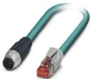
Network cable, Ethernet CAT5 (1 Gbps), 8-position, Plug straight M12 / IP67, coding: A, on Plug straight RJ45 / IP20, cable length: 3 m
