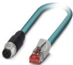
Assembled Ethernet cable, CAT5e, shielded, 2-pair, AWG 26, stranded (7-wire), RAL 5021 (aqua blue), M12 plug to RJ45 plug/IP20, line, length 1 m
