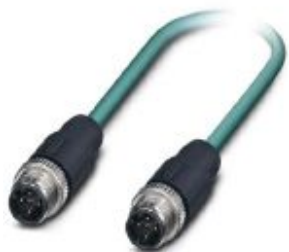
Assembled Ethernet cable, CAT5e, shielded, 2-pair, AWG 26 stranded (7-wire), RAL 5021 (sea blue), M12 plug to M12 plug, line, length 1 m
