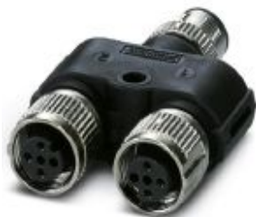
Y distributor, 3-position, unshielded, Plug straight M12 SPEEDCON, coding: A, on Socket straight M12 SPEEDCON, coding: A and Socket straight M12 SPEEDCON, coding: A, with 3 LEDs
