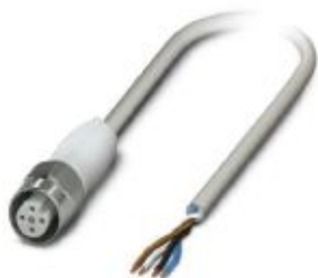
Sensor/actuator cable, 4-position, PP-EPDM halogen-free, gray RAL 7035, free cable end, on Socket straight M12, coding: A, cable length: 1.5 m, Hygienic design, with high-grade steel knurl
