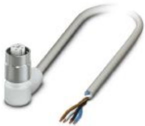
Sensor/actuator cable, 4-position, PP-EPDM halogen-free, gray RAL 7035, free cable end, on Socket angled M12, coding: A, cable length: 10 m, Hygienic design, with high-grade steel knurl
