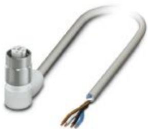
Sensor/actuator cable, 4-position, PP-EPDM halogen-free, gray RAL 7035, free cable end, on Socket angled M12, coding: A, with 3 LEDs, cable length: 1.5 m, Hygienic design, with high-grade steel knurl
