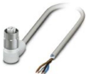
Sensor/actuator cable, 4-position, PP-EPDM halogen-free, gray RAL 7035, free cable end, on Socket angled M12, coding: A, with 3 LEDs, cable length: 5 m, Hygienic design, with high-grade steel knurl
