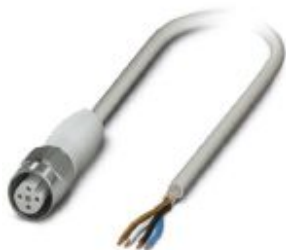
Sensor/actuator cable, 4-position, PP-EPDM halogen-free, gray RAL 7035, shielded, free cable end, on Socket straight M12, coding: A, cable length: 5 m, Hygienic design, with high-grade steel knurl
