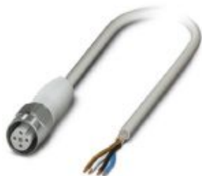
Sensor/actuator cable, 4-position, PP-EPDM halogen-free, gray RAL 7035, shielded, free cable end, on Socket straight M12, coding: A, cable length: 10 m, Hygienic design, with high-grade steel knurl
