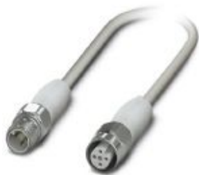
Sensor/actuator cable, 4-position, PP-EPDM halogen-free, gray RAL 7035, shielded, Plug straight M12, coding: A, on Socket straight M12, coding: A, cable length: 3 m, Hygienic design, with high-grade steel knurl
