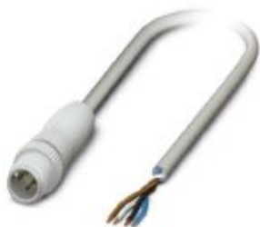
Sensor/actuator cable, 4-position, PP-EPDM halogen-free, gray RAL 7035, Plug straight M12, coding: A, on free cable end, cable length: 3 m, Hygienic design, with plastic knurl
