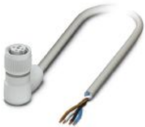
Sensor/actuator cable, 4-position, PP-EPDM halogen-free, gray RAL 7035, free cable end, on Socket angled M12, coding: A, cable length: 10 m, Hygienic design, with plastic knurl
