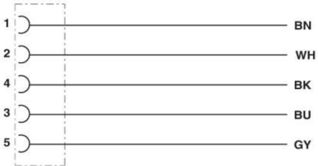
Contact assignment of the M12 socket
