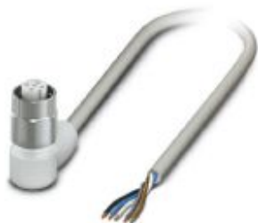
Sensor/actuator cable, 5-position, PP-EPDM halogen-free, gray RAL 7035, free cable end, on Socket angled M12, coding: A, with 3 LEDs, cable length: 5 m, Hygienic design, with high-grade steel knurl
