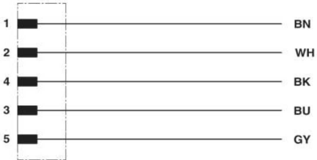
Contact assignment of the M12 plug
