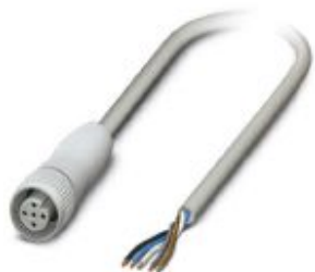
Sensor/actuator cable, 5-position, PP-EPDM halogen-free, gray RAL 7035, free cable end, on Socket straight M12, coding: A, cable length: 3 m, Hygienic design, with plastic knurl
