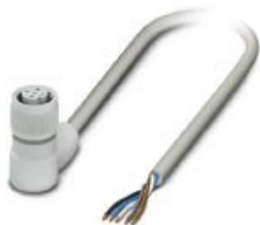
Sensor/actuator cable, 5-position, PP-EPDM halogen-free, gray RAL 7035, free cable end, on Socket angled M12, coding: A, cable length: 5 m, Hygienic design, with plastic knurl
