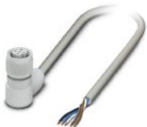
Sensor/actuator cable, 5-position, PP-EPDM halogen-free, gray RAL 7035, free cable end, on Socket angled M12, coding: A, with 3 LEDs, cable length: 10 m, Hygienic design, with plastic knurl
