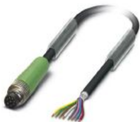
Sensor/actuator cable, 8-position, PUR halogen-free, black-gray RAL 7021, shielded, Plug straight M8, on free cable end, cable length: 10 m
