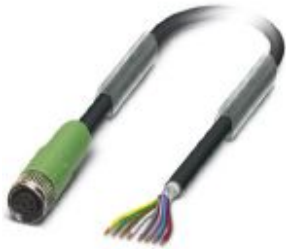
Sensor/actuator cable, 8-position, PUR halogen-free, black-gray RAL 7021, shielded, free cable end, on Socket straight M8, cable length: 10 m
