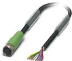
Sensor/actuator cable, 8-position, PUR halogen-free, black-gray RAL 7021, free cable end, on Socket straight M8, cable length: 3 m
