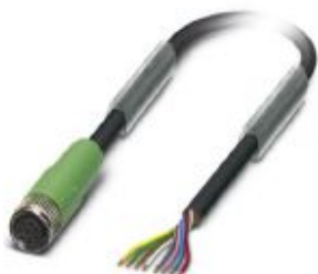
Sensor/actuator cable, 8-position, PUR halogen-free, black-gray RAL 7021, free cable end, on Socket straight M8, cable length: 5 m
