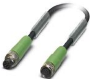
Sensor/actuator cable, 8-position, PUR halogen-free, black-gray RAL 7021, Plug straight M8, on Socket straight M8, cable length: 1.5 m
