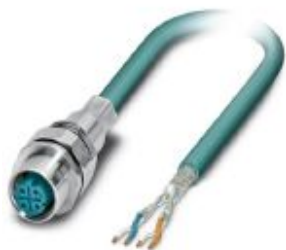
Assembled Ethernet cable, CAT5e, shielded, 2-pair, AWG 26 stranded (7-wire), RAL 5021 (water blue), M12 flush-type socket, front/screw mounting with M16 thread on free conductor end, line, length 5 m
