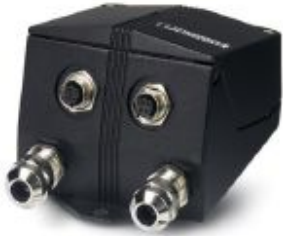
Terminal outlet M12 IP65/67, 2 slots 4-pos. D-coded, with protective plugs, 2 cable entries
