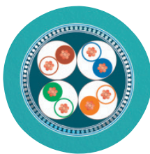
Cable cross section
